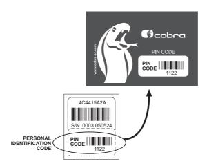
We advise you to stick the PIN CODE, which may be found on the rear of the control unit, adhesive label on to the PIN CODE CARD.
