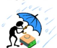
**Although designed to be resistant to water ingress (IPX5), this electronic equipment might be damaged by steam cleaning / high pressure washing. Never direct the jet at the unit and protect it to prevent water infiltration.**
